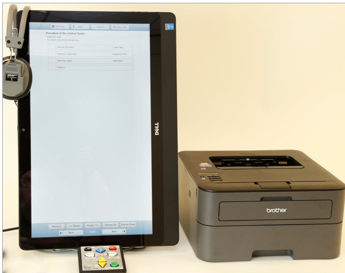
Figure 5-1. An example ClearAccess setup
